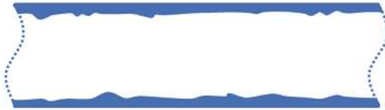
Figure 3.3 – Pipe wall Interior Roughness
