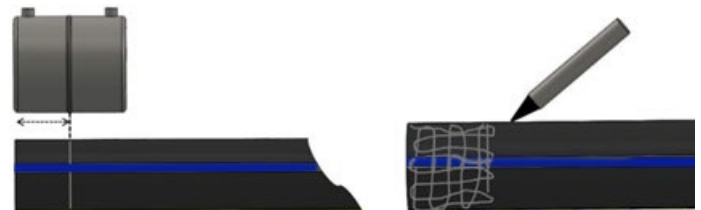
Figure X-c- Measure and mark Stab Depth
