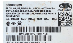
Figure IX-a – Barcode with Fitting Information
