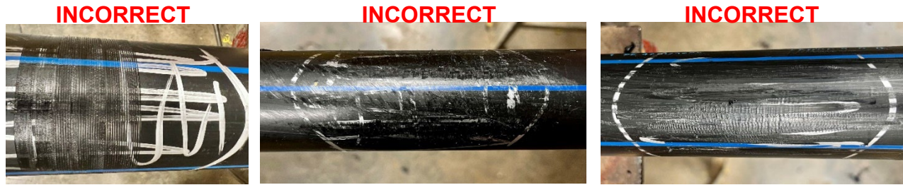
Figure X-p - Incorrect Peeling! Improper surface preparation: Not enough material removed, marks still visible
