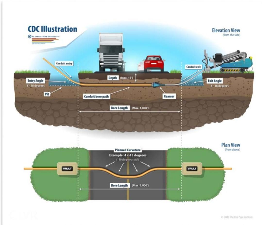
**Figure 1 - Schematic of Typical Mini-HDD Installation**
