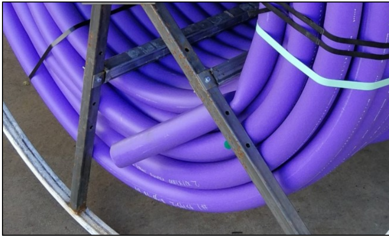
Figure 4: End of a coil of conduit showing deformation
