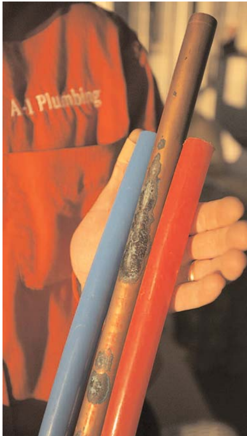
Copper pipes with pinholes leaks were replaced with a long-life PEX system
