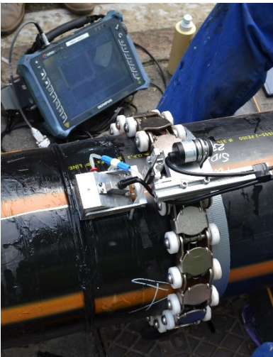
Phased array ultrasonic inspection of butt fusion joint in PE gas pipe using TWI's PolyTest system. Photo courtesy of TWI Ltd
