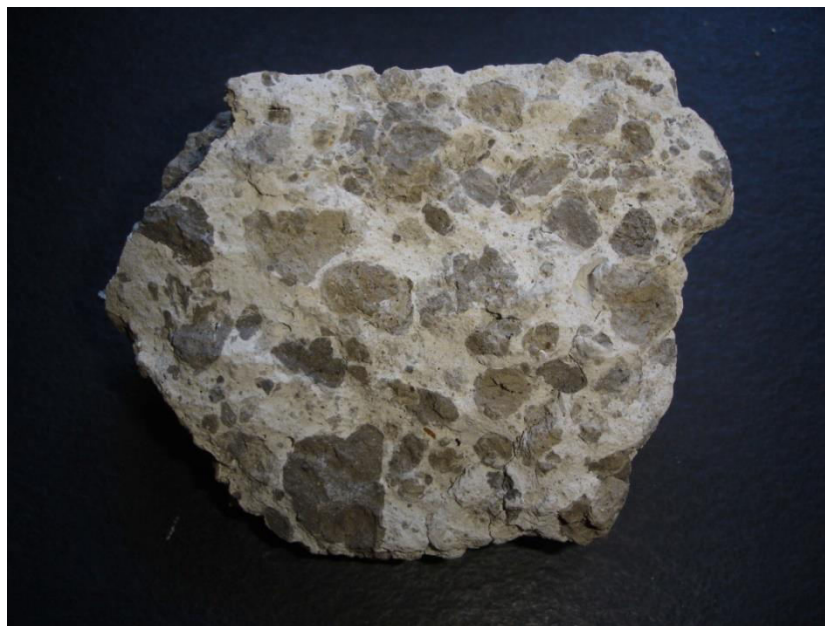
Figure 5 Chunk of flowable fill made using insitu clay soil
