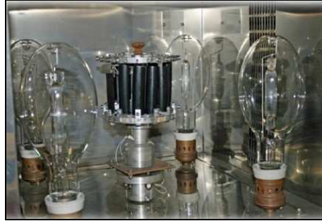
Figure II: 12/24 SEPAP cell, photo-thermo-oxidative accelerated ageing
