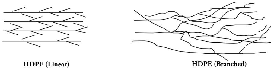
**Figure 1-2: Schematic of Linear and Branched Arrangements**
