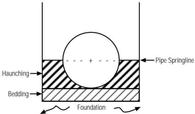
Additional attention should be given to backfill placement and compaction around pipe connections at manholes, catch basins, fittings, and other structures. Since it can be difficult to work in these areas, the backfilling process is often neglected. This can lead to non-uniform settlement or product damage. As a precautionary measure in critical applications, a pipe joint can be made close to the manhole to help accommodate differential settlement, as shown in figure 6A (following page).
