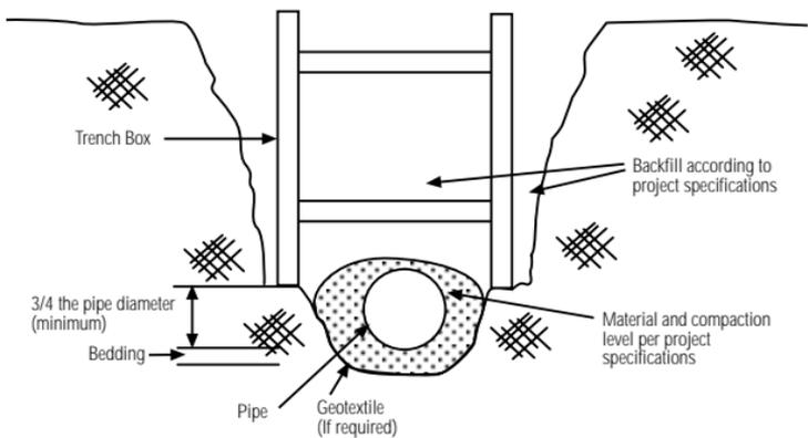
Subtrench installations also make it easier to use a geotextile around the backfill if it is required by the project specifications. The subtrench can be lined with the geotextile, and then wrapped around the pipe and backfill so that it overlaps slightly.
