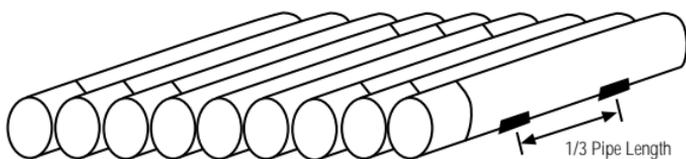
A reasonable amount of care in handling the pipe should be taken during stockpiling. The pipe should not be dropped, dragged, or bumped against other pipe or objects, or climbed on. Stockpile heights should be limited to approximately 6' (2 m) so that the pipe can be handled easily and safely manually.
