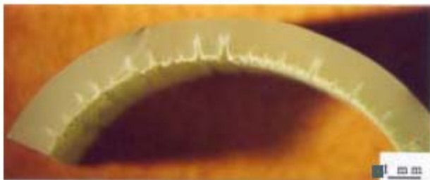
Figure 3: Radial Crack Growth in a PEX Pipe Material
