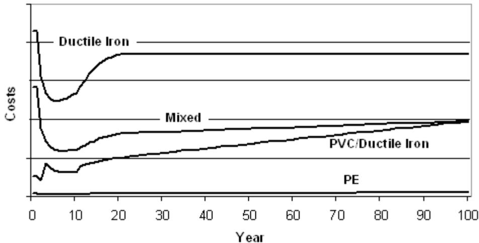
**Fig. 3. Whole of life costing simulation (excluding installation costs) for a medium sized network<sup>2</sup>**
