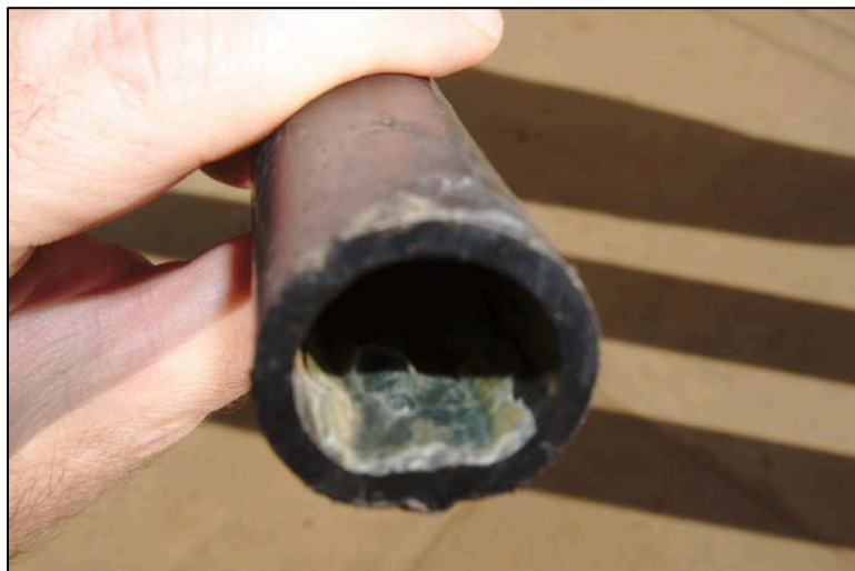
Figure 7: HDPE water pipe with melted material deposits
