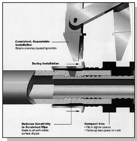
Figure 5 – External Compression Ring style coupling
