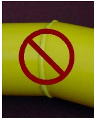
Figure A 1: Visually unacceptable mitered joint.
