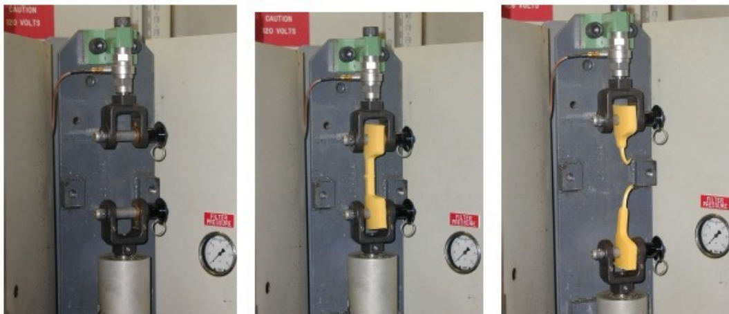
Figure 2: Typical McSnapper™ test set-up and testing progression of a typical PA12 test specimens at an average speed of 6 in/s.
