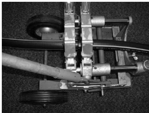
Figure A 2: Coiled pipe with residual curvature correctly positioned in the butt fusion machine.
